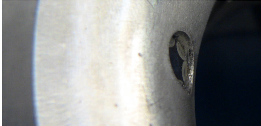
Figure 5: Example of Sensor Tip that is Not Sufficiently Deep
