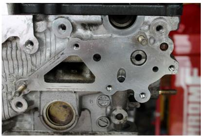
Remove the 2 studs from the head, use the double nut trick.
