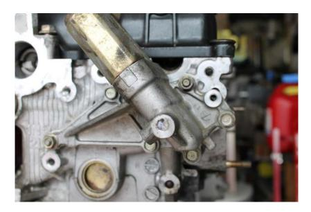
Clean any excess gasket off both the solenoids and the head surfaces.
