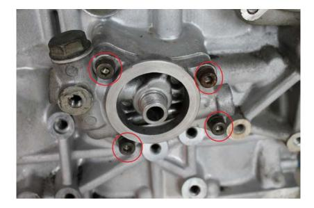
Once the old oil filter block has been removed this is what you are left with, be very careful not drop anything into the oil holes.
