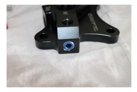
If your using the oil block to run a VVL feed then install the AN6 ORB adapter. If you do not require the VVL feed port then use the AN6 ORB plug to block if off. No PTFE tape is require, just use the supplied o-rings as pictured below. Apply a small amount of oil to the o-rings prior to installing.
