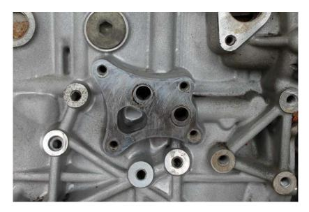
Once the old oil filter block has been removed clean any oil build-up etc off the aluminium, otherwise the o-rings will not seal properly.
