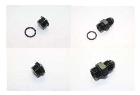
This oil block has been setup for an SR20det so the VVL feed was not required. Again, do not over tighten the plug or adapter.
