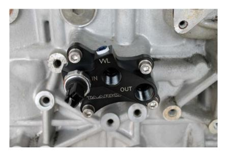
Install the supplied o-rings onto the fittings as shown below.
