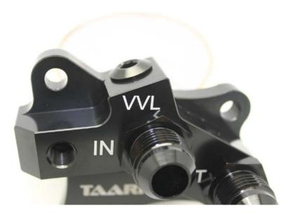
Use an aluminium shifter, or if you do not have access to an aluminium shifter a rag and normal shifter will do the trick. This is to protect the fittings anodising from scratches.
