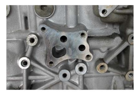
If you are not planning on installing a gauge sensor or similar into the spare 1/8" NPT port then use the supplied plug with some PTFE plumbers tape to block if off. 3 turns of tape will be fine. Remove any excess tape before installing the plug.
