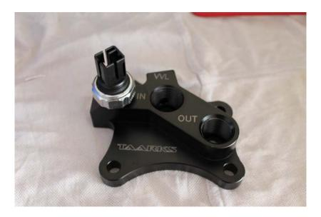
Apply a small amount of engine oil to the supplied o-rings and insert them into the rear of the oil block. The oil will help hold them in place.
