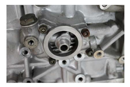
Remove the old oil filter block by removing the 4 allen key bolts using a 6mm allen key.
