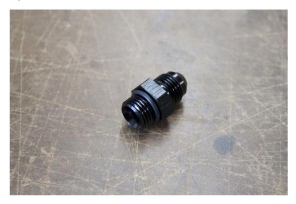
Install the fitting into the oil block. Do not use thread sealant.
