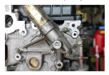
Clean any excess gasket off the head surface.
