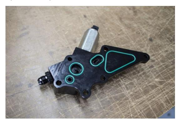
Using the supplied M6 bolts, washers and spring washers install the solenoid block onto the head.
