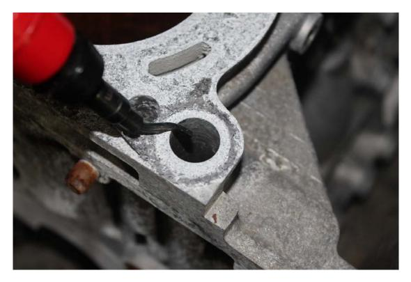
Thread an M6 bolt completely into the oil drain plug. Apply a lubricant to the o-rings and the oil drain hole (engine oil works well)
