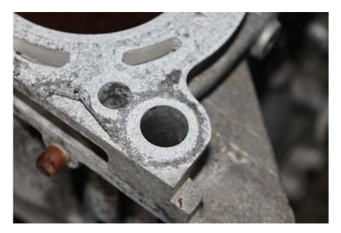
De-burr the top edge of the hole to remove any sharp edges. Failure to do this may damage the o-rings.
