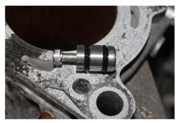
Using a press, slowly press the plug into the engine block. Be sure to check the o-rings do not get damaged.
