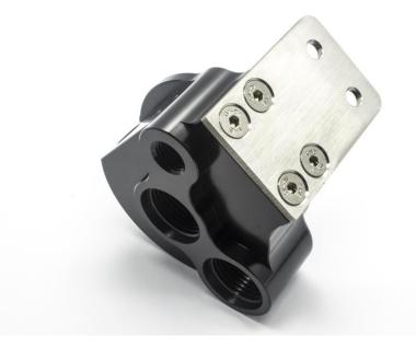
The aluminium housing has a M12x1.5 threaded port to accept a temperature sensor. If you are not using a temperature sensor install the supplied plug as shown below.
