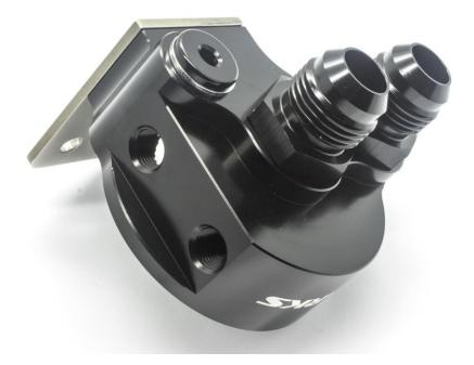
The aluminium housing has 2x 1/8" NPT ports for temperature and pressure sensors. If you plan on using a pressure sensor the preferred port is lower port in the picture below, this will measure oil pressure after the filter.
