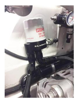
Please note that oil will only flow in one direction through an oil filter due to the internal check valve. Ensure the lines are plumbed correctly during installation. Oil should flow from the engine or oil cooler to the outside of the oil filter and return to the motor from the center of the oil filter.
