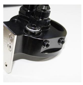
The port circled below is an option oil drain port. When mounted with the oil filter facing up, a fitting and hose can be connected to this port so when the oil filter is removed any excess oil in the filter will drain down the hose into the oil drain pan. When the oil filter is mounted upside down this port can be left unused or blocked off. The thread size is  $\frac{1}{4}$ " NPT.
