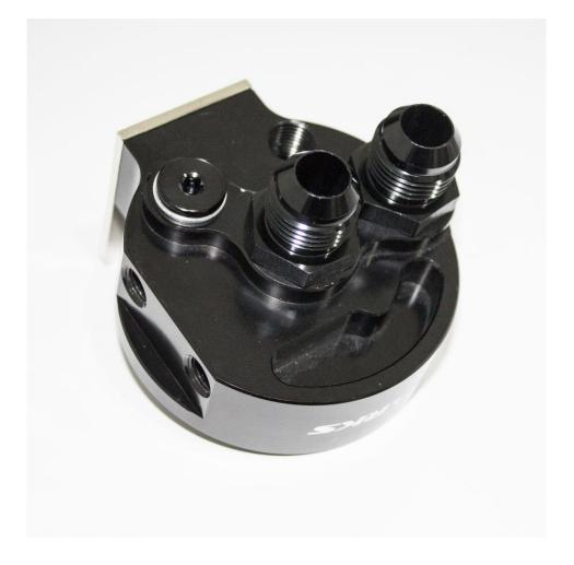
The aluminium housing has 2x 1/8" NPT ports for temperature and pressure sensors. If you plan on using a pressure sensor the preferred port is lower port in the picture below, this will measure oil pressure after the filter.
