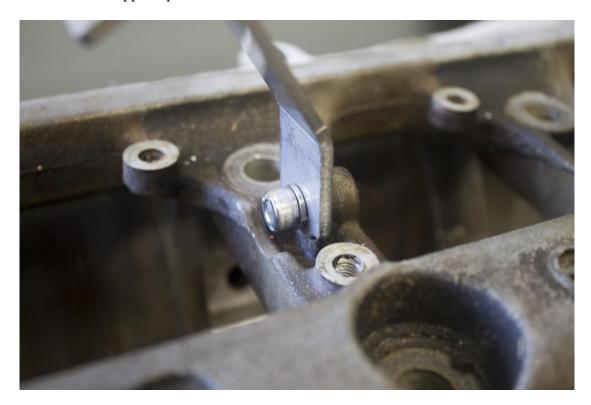
Install the supplied o-ring into the flange of the pick up.
