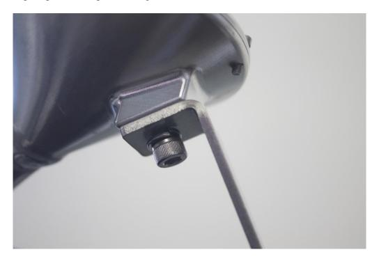
The bolts can now be tightened. Starting with the 2xM8 bolts holding the pick up to the oil pump, followed by the M6 bolt holding the bracket to cradle and lastly the M6 bolt holding the bracket to the pick up.
