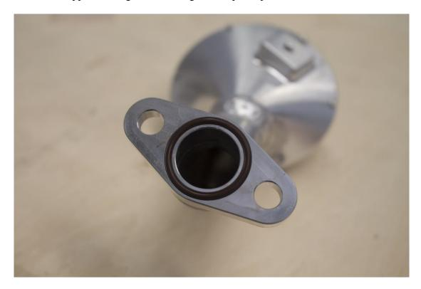
Using the supplied M8x20mm bolts and spring washers mount the pick up onto the oil pump, be careful that the o-ring does not come out of it's groove. Do not tighten the bolts just yet, nip them up.
