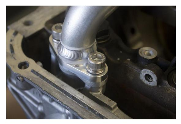
Due to the welding process and nissan's machining of the oil pump/cradle you may need to slightly bend the stainless steel bracket to line up with the mounting hole on the pick up.
