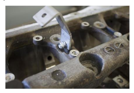
Once the bolt starts to compress the spring washer gently push the bracket down while you continue tightening the bolt. Nip the bolt up (do not tighten just yet).
