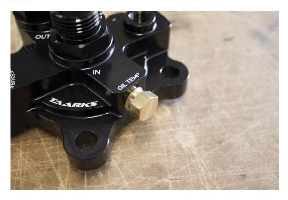
The oil blocks have 2 spare 1/8" NPT ports for gauges etc, if these are not required installed the supplied plugs, these will require thread tape.
