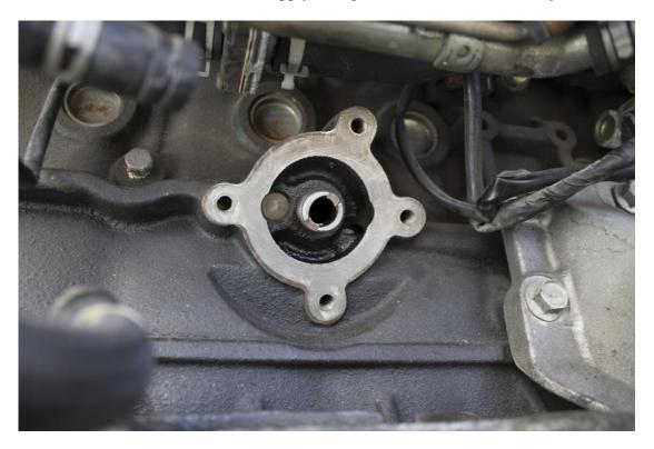
Install the supplied o-rings as pictured below. Take care when installing the small o-ring.
