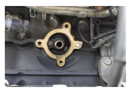
Remove the old gasket and ensure the surface is nice and clean. At this stage you can remove the M8 stud towards the front of the motor, this is not 100% required, you can re-use the standard nut, but we do supply enough stainless bolts so that they all match.
