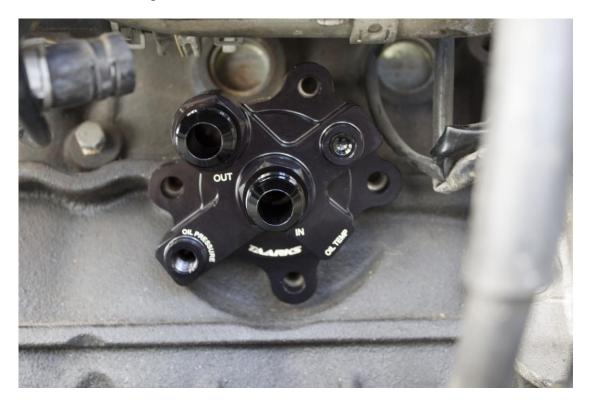
Install the supplied M8 stainless steel bolts and spring washers.
