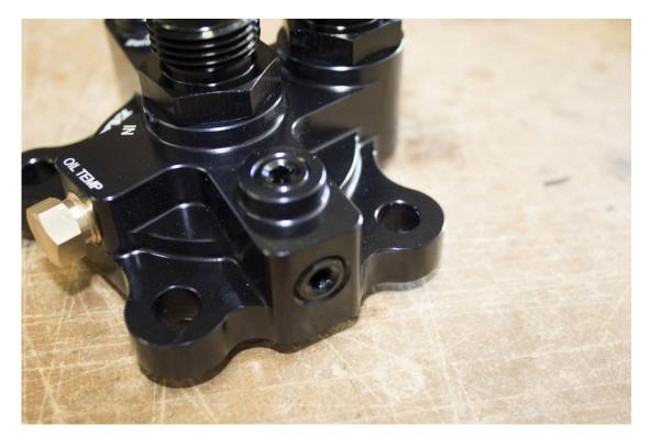
Lubricate the 2 o-rings on the rear of the oil block and also lubricate the stud on the engine block. Press the oil block over the stud on the engine block and gently rotate back and forth to help it on.
