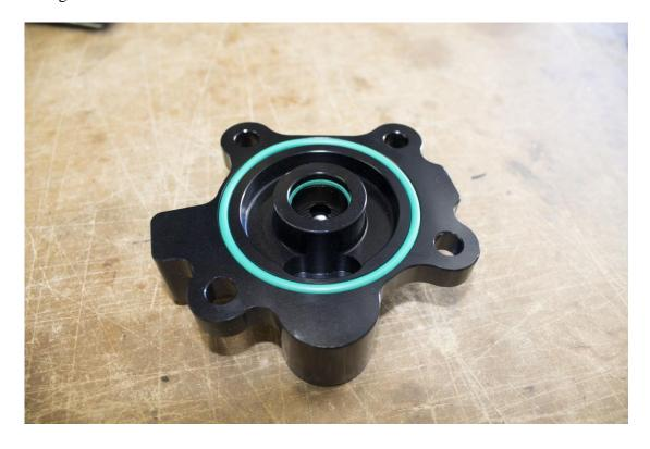
Install the o-rings onto the AN10 fittings.
