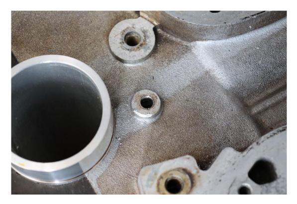
Use a M7x1 tap to thread the hole, ensure the tap is perfectly straight.
