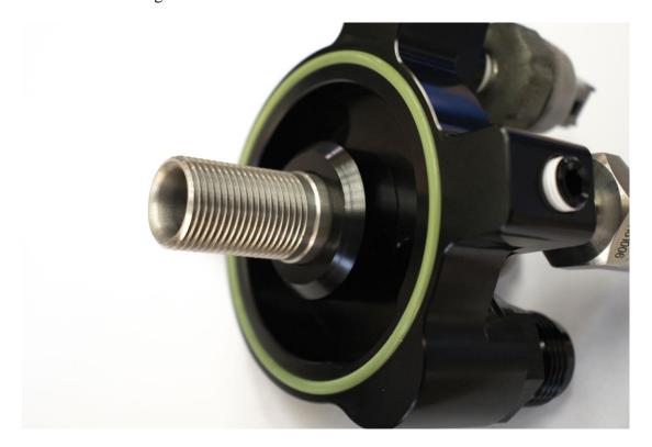
Install the oil block onto the engine block ensuring the tab on the side slides over the dowel on the block.
