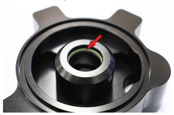
Install the 70x3mm Viton o-ring into the oil block as shown below.
