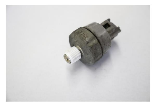
Install the factory oil pressure sensor into the oil block port labelled "Oil Switch 1/8 BSPT" as shown below.
