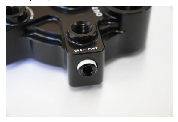
The oil block has a M12x1.5mm port for an oil temp sensor, install a sensor or use the supplied plug and washer to block the port if a sensor is not being used.
