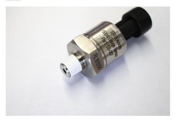
Install the sensors into any unused 1/8" NPT ports. (Note: The side facing 1/8" NPT port is not recommended for large sensors due to clearance issues with the A/C compressor)
