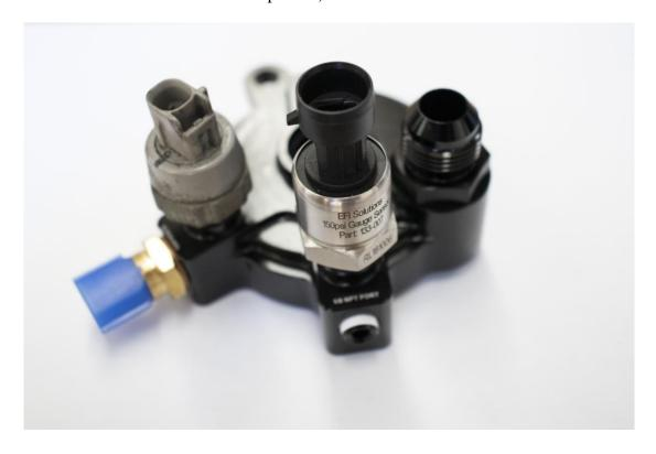
Apply a light coating of oil to the o-ring, shaft and threads of the stainless steel mounting bolt as shown below.
