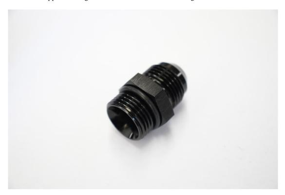
Apply a small amount of engine oil to the o-ring and threads of the AN10 ORB fitting and install it into the oil block. Use a long reach 1" socket and torque to 30-36 ft.-lbs. ensure there is no damage to the flare surface.
