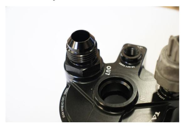
Apply Teflon tape or liquid thread sealant to the threads of any additional 1/8" NPT sensors.
