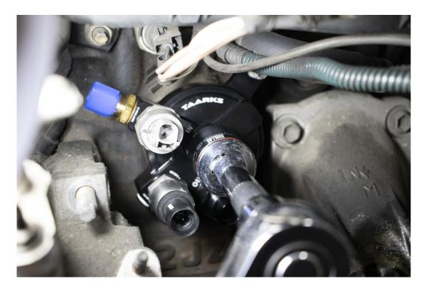
Connect any electrical connectors and AN lines to the block, prime the oiling system by cranking the engine with the ignition system disabled and check for leaks.
