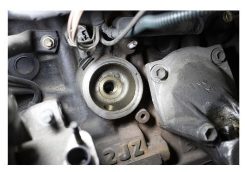
Install the 19x3mm Viton o-ring into the oil block as shown below.
