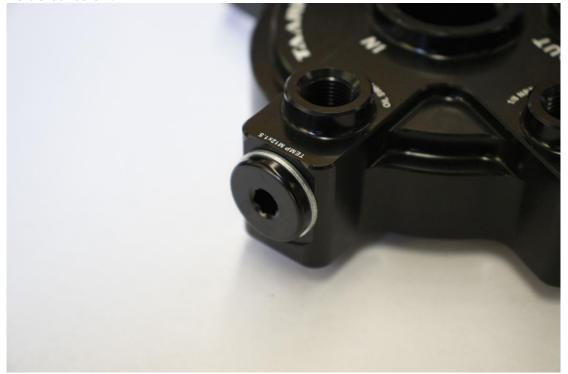
Apply Teflon tape or liquid thread sealant to the threads of the factory oil pressure sensor.
