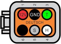
Pin 1/Red = 12v + (Filtered from ECU)Pin 2/Black = Sensor GND (from ECU) Pin 3/Green = Trigger (North Pole) Pin 4/White = Home/Sync (South Pole) Pin 5/Raw = Shield
