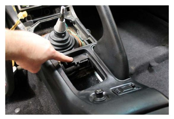
Remove the red backing off the double sided tape located on the underside of the cup holder. Be careful not to pull the tape off the cup holder.
