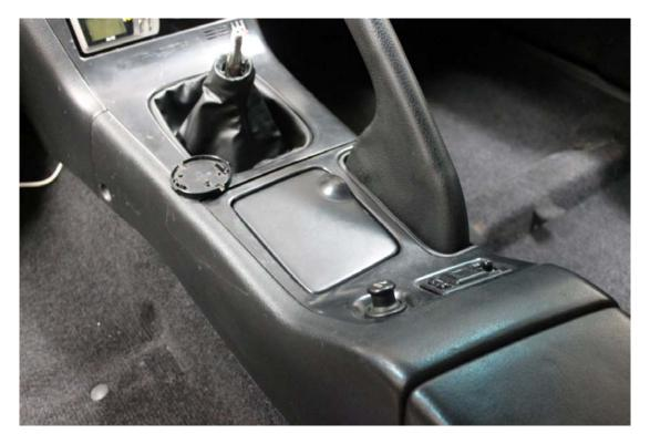
Unclip and remove the gear shifter surround.
