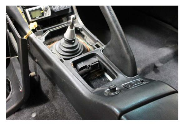
Clean the area shown in the photo below with an alcohol based product. (metho, acetone, prepsol, etc) do not use an oil based cleaner (turps, petrol, etc) be carful to keep the cleaner away from any of the interior except the part shown in the photo below. If you skip this step the supplied double sided tape will not hold.
