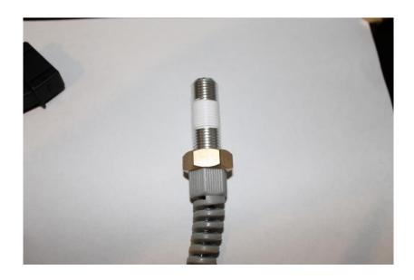
Install the hall sensor into the sensor holder. Leave about 10mm of the sensor sticking out. Do not tighten the nut just yet. Apply some engine oil to the o-ring.
