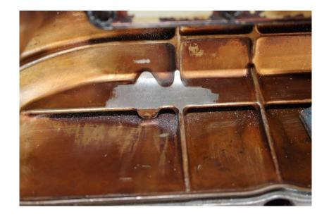
Ensure any metal filings are removed before re-fitting the rocker cover.
