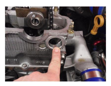
Once the plug has been removed use some 1000 or 1200 grit sand paper to clean any residue out of the hole. Place a rag at the back to stop any dust or debris from falling into the motor.
