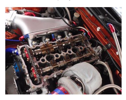
Set the motor to TDC on cylinder one. The lobes on the camshafts for cylinder one will face away from each other.
