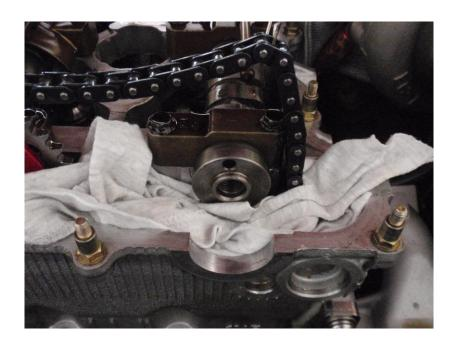
Install the supplied dowel pin into the exhaust camshaft. Note that the tapered end goes in first, as pictured.
