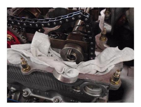
Remove the 30mm welsh plug from the front of the head. The plug needs to be pushed from the rear. This can be done very gently with large screwdriver (or similar) and a rubber mallet.
