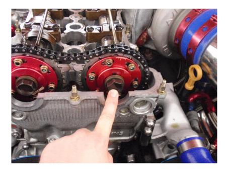
Remove the exhaust cam gear and support the chain. Do not let the chain drop.
