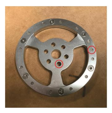
Install the supplied hall wheel. Gently tap the hall wheel onto the dowel.
