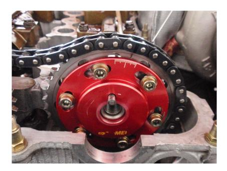
The newly designed hall wheels now have 6 dowel pin locations. This is so you can change when TDC offset of the home signal occurs. Some ECU's require the home/sync signal to occur in a particular window in the engine cycle. If you plan to use the provided ECU settings at the end of this guide you will need to use the dowel hole circled below. Make sure the home magnet (circled) is as pictured in the photo.
