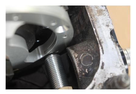
Using the supplied cam washer gently tighten the bolt to pull the hall wheel up against the cam gear.
