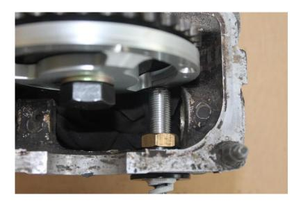
Install the CAS block off plug using the suppled stainless bolts. A small amount of oil on the o-rings will help it slide in.
