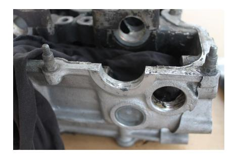
Once the plug has been removed use some 1000 or 1200 grit sand paper to clean any residue out of the hole. Place a rag at the back to stop any dust or debris from falling into the motor.
