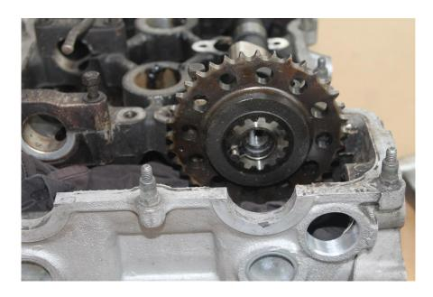
The newly designed hall wheels now have 6 dowel pin locations. This is so you can change when TDC offset of the home signal occurs. Some ECU's require the home/sync signal to occur in a particular window in the engine cycle. If you plan to use the provided ECU settings at the end of this guide you will need to use the dowel hole circled below. Make sure the home magnet (circled) is as pictured in the photo.
