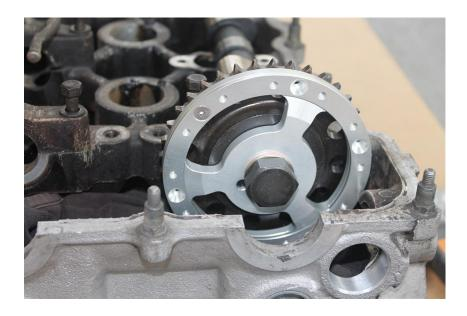
PLEASE NOTE: We have modified the design, this kit now uses the factory cam bolt and we now supply a spacer to emulate the factory CAS gear.
