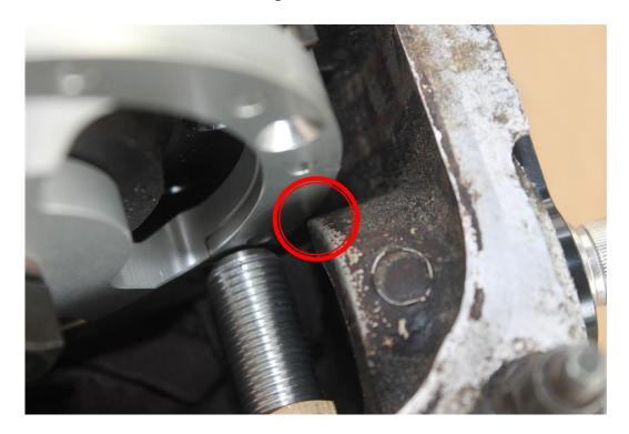
Using the factory cam bolt washer and supplied flanged bolt gently tighten the bolt to pull the hall wheel up against the cam gear.
