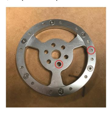
Install the supplied hall wheel. Gently tap the hall wheel onto the dowel if needed.
