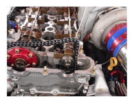
Remove the worm gear from the cam gear.
