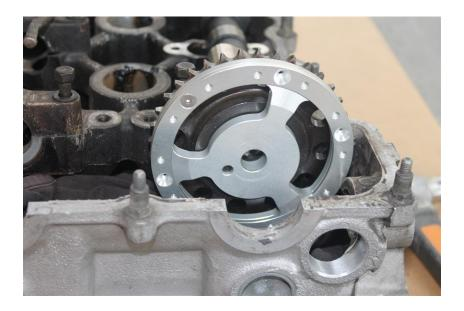
Check for any clearance issues. Some aftermarket cam gears may push the hall wheel further forward, some material may need to be removed from where the old CAS mount protrudes into the head.
