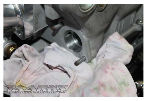
Once the tensioner has been removed push down on the timing chain between the cam gears. You may notice one or both of the cam gears move, this is normal.
