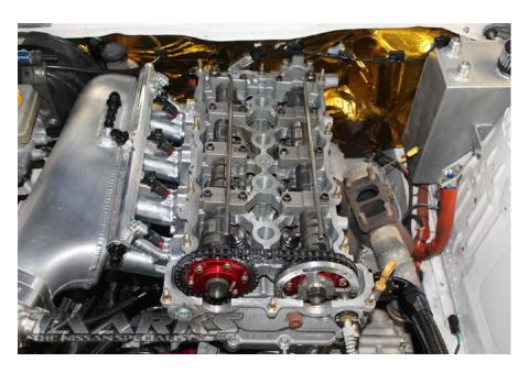
Remove the timing chain tensioner by removing the 2 10mm nuts, slowly back each nut off evenly as the tensioner is spring loaded.
