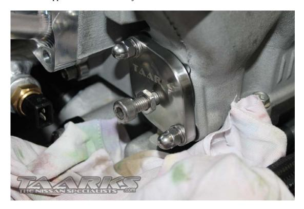
Slowly wind the tensioner bolt in. You will see the slack between the cam gears starting to go away
