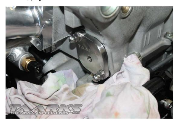
Install the supplied M8 bolt with the jam nut into the tensioner.
