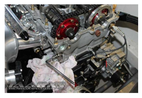
Using a ruler keep checking the tension on the chain. By gently pressing down and pulling up on the chain with a small amount of force, you want around 6mm of slack.
