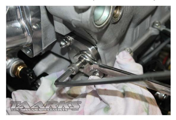
Turn the motor over by hand ensuring everything is operating correctly.
