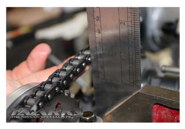
Once the correct tension has been set, use the jam nut to lock the tensioner in place.
