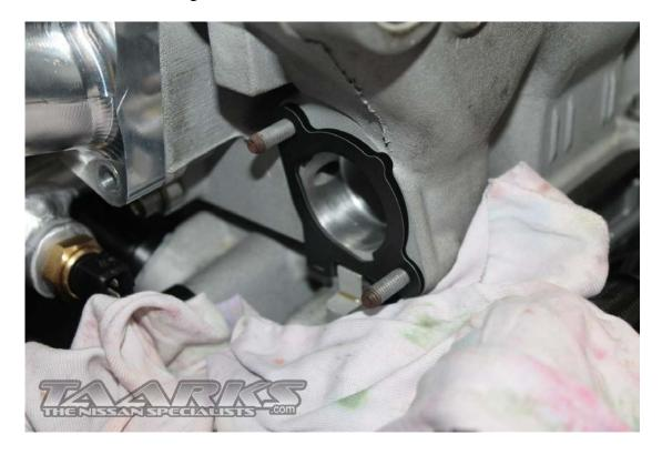
Slowly insert the new tensioner and ensure the slot in the tensioner shaft mates up to the chain guide correctly. This can be visually verified by looking down the chain valley. Failure to do so will cause engine damage. Once in place install the supplied flat washer, spring washer and dome nuts in that order.
