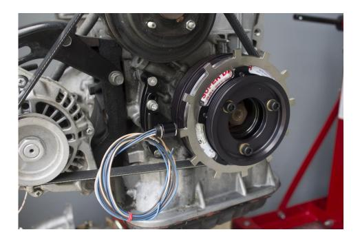
Continue to wind the sensor in until you reach an air gap of between 1mm-1.5mm. Now tighten the lock nuts to keep the sensor in place. A small amount of blue Loctite can be used.
