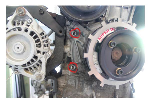
Using the supplied 2x M6x25mm cap screws, split washers and flat washers assemble the sensor mount as shown below. Also thread the sensor into the mount and thread a locking nut either side.
