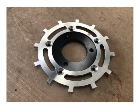
Install the 5x M6 countersunk bolts to secure the trigger wheel onto the hub. Use red high strength Loctite on the threads. Use a 4mm allen key to tighten.
