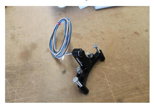
Install the sensor bracket onto the engine using the supplied M6x50mm counter sunk bolts.
