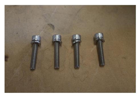
Using the M6x35mm bolts install the bracket onto the rocker cover. Be careful to not knock any of the spacers. A 5mm allen key is required.
