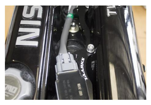
Install the 2<sup>nd</sup> coil using the supplied M6x20mm bolts and M6 spring washers. A 5mm allen key is required.
