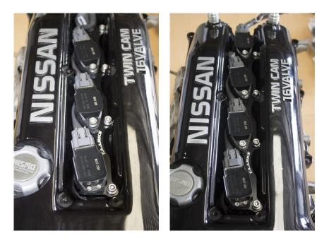
Note: It is recommended to run Resistor type spark plugs with these coils, running non resistor plugs can damage the coils.
