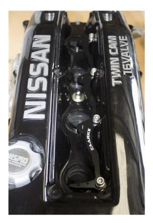
On each of the coils use a small amount of the supplied dielectric grease on the inside of the coil boot where the spark plug enters, this helps the boot slide on and off the spark plug easier. Install the pre-modified coil into the #1 spark plug hole.
