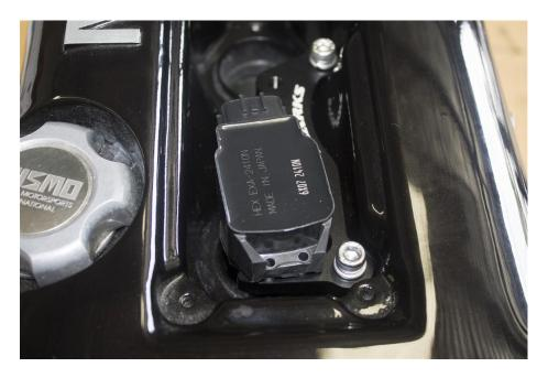
Using the supplied M3x16mm bolts and M3 spring washers bolt the coil down to the bracket. A 2.5mm allen key is required.
