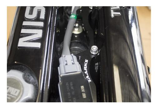
Install the 2<sup>nd</sup> coil using the supplied M6x20mm bolts and M6 spring washers. A 5mm allen key is required.
