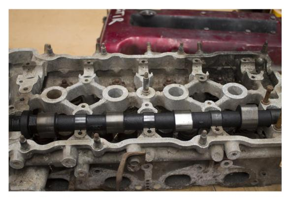
Remove the centre rocker cover bolt using a 10mm spanner.
