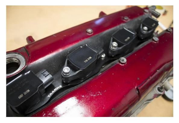
Using a 5mm allen key tighten the centre mounting bolt.
