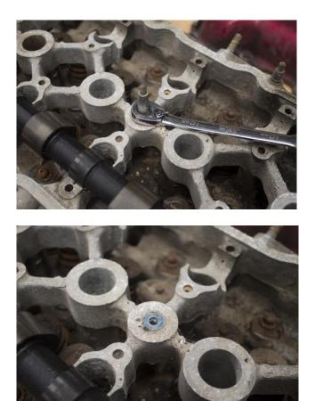
Re-install the rocker cover and insert the supplier rocker cover washer.
