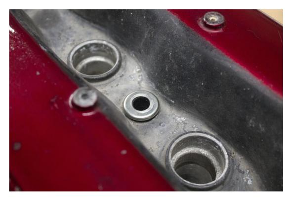
Install the supplied coil bracket mount.
