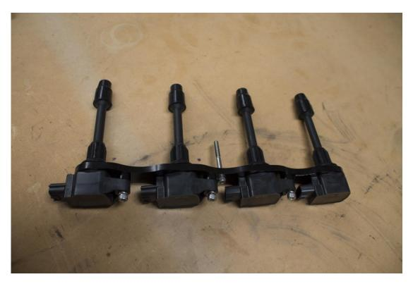
On each of the coils use a small amount of the supplied dielectric grease on the inside of the coil boot where the spark plug enters, this helps the boot slide on and off the spark plug easier. Install the coil packs into the rocker cover by gently pushing the coils down into the spark plug holes. Guide the centre M6 bolt into the coil bracket mount.
