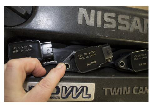
Once the #2 coil has been rotated out of the way you can install the connector onto the #1 coil, rotate the #2 coil back into place and gently push down on the connector and mounting tab rocking back and forth until the coil is seated once more.
