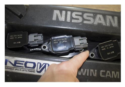
The same process is to be followed for the #4 coil to install the connector onto the #3 coil. The connector for the #4 coil can be installed without moving any of the other coils.
