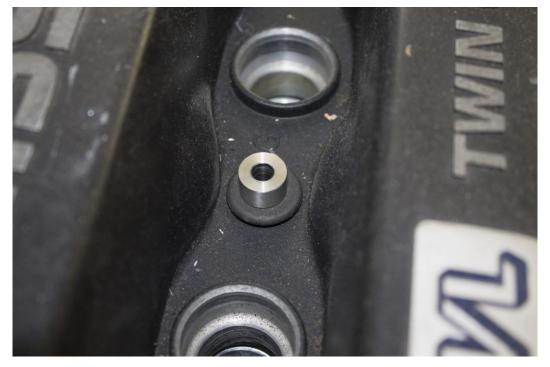
On each of the coils use a small amount of the supplied dielectric grease on the inside of the coil boot where the spark plug enters, this helps the boot slide on and off the spark plug easier. Install the complete coil kit by lining the coil boots up with the spark plug wells and gently pushing down. Ensure the centre mounting bolt goes into the stainless mount in the centre of the rocker cover.
