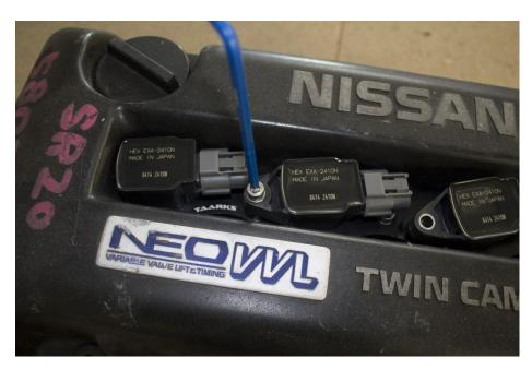
Note: It is recommended to run Resistor type spark plugs with these coils, running non resistor plugs can damage the coils.
