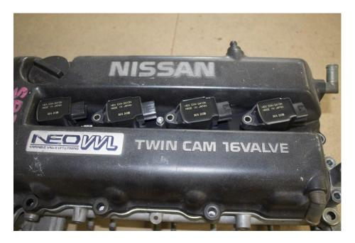
Gently rock the #2 coil by holding onto the connector end and mounting end. Gently pull up while rocking the coil. You will feel the coil pop up slightly, this will allow you to rotate the coil as shown below.
