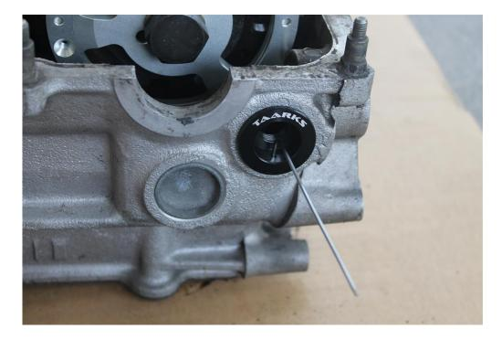
Wind the hall sensor into the holder so the tip of the sensor protrudes around 3mm, wind the supplied nut onto the sensor.
