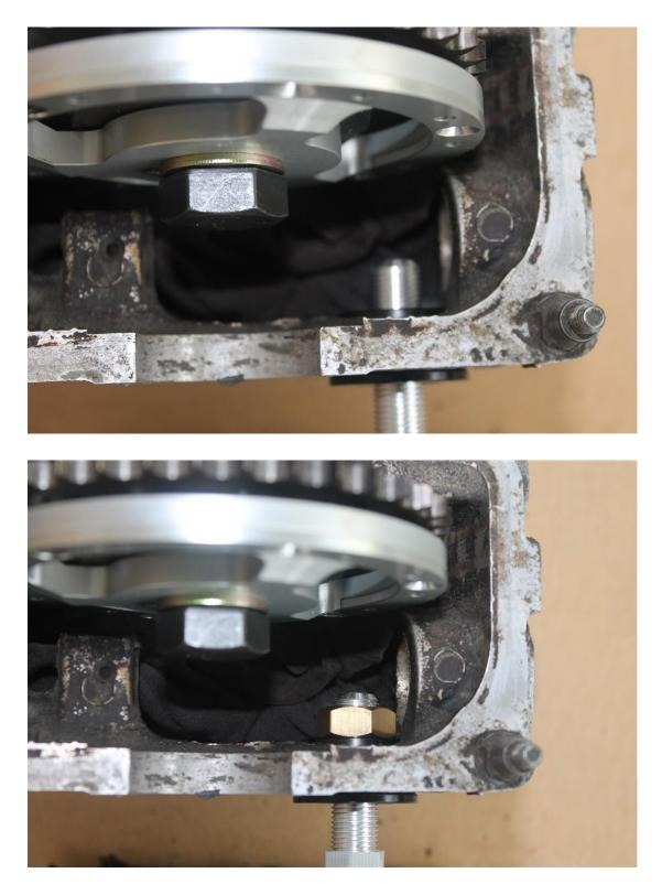
Wind the sensor in until the end of the sensor is 1mm away from the hall wheel. Use a feeler gauge to check the distance, rotate the engine and check the distance at several points around the hall wheel. (This distance may need to be adjusted once the motor is up and running, a gap no smaller than 0.5mm may be used). Once the sensor is in position apply some Loctite to the thread of the sensor just after the holder and wind the nut hard up against the holder and tighten.
