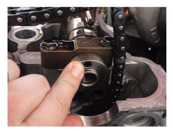
Place rags under the camshaft in case you drop the dowel.
