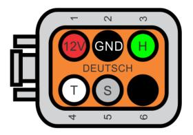
Pin 1/Red = 12v+ (Filtered from ECU) Pin 2/Black = Sensor GND (from ECU) Pin 3/Green = Home/Sync Pin 4/White = Trigger Pin 5/Raw = Shield Pin 6 = Not Used
