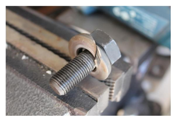
Use a cold chisel or flat blade screw diver and break the washer off. Once removed you will be left with just the bolt.
