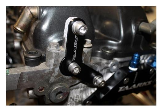
On the rocker cover a small part of the internal fins need to be ground down to clear the hall wheel.
