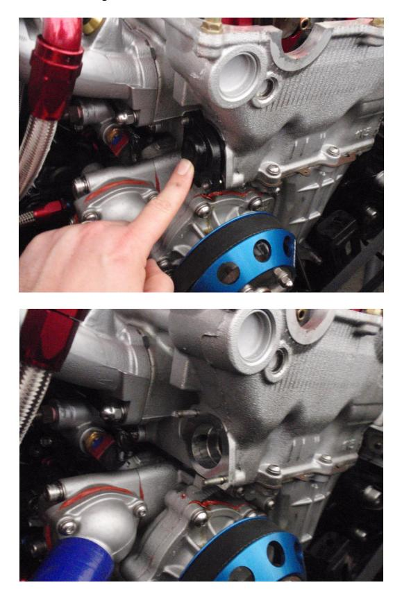
Remove the timing chain tensioner.
