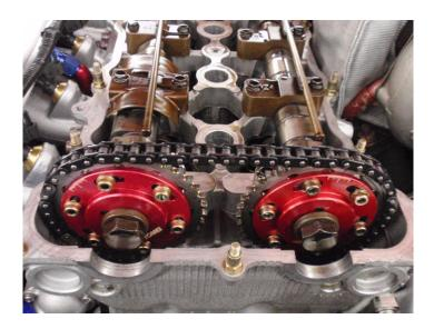
Mark the timing chain with a marker at the timing marks on the cams gears.
