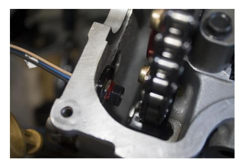
If you are using the P11 rocker cover a small part of the internal fins need to be ground down to clear the hall wheel. (P12 rocker covers do not need this done)
