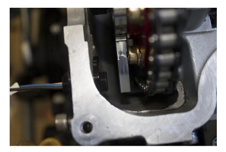
Install the locking nut onto the sensor, place some rags under the sensor in case the nut drops.
