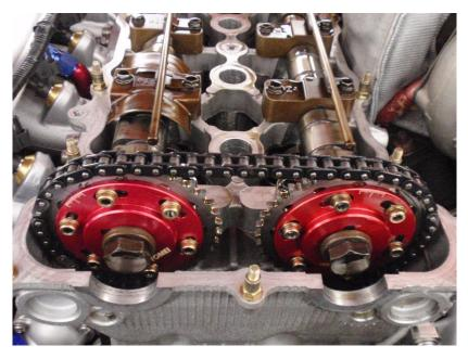
Mark the timing chain with a marker at the timing marks on the cams gears.
