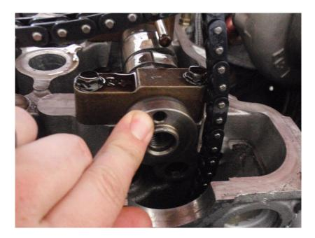
Place rags under the camshaft in case you drop the dowel.
