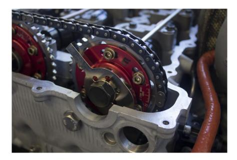
Check that you have clearance between the trigger plate and any of the adjustable cam gear bolts, if necessary machine down the bolt heads to provide a small amount of clearance.
