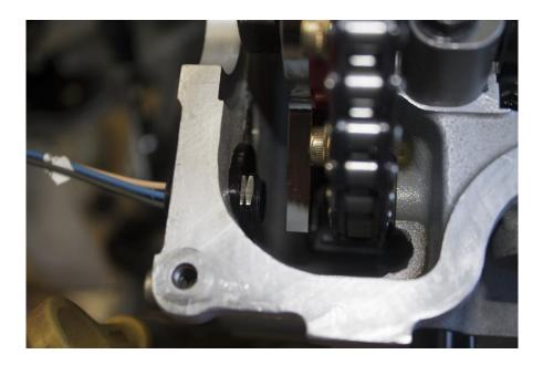
Wind the motor over so the trigger finger is in front of the sensor. Wind the sensor in so there is 1mm air gap.
