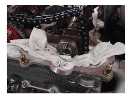
Remove the 30mm welsh plug from the front of the head. The plug needs to be pushed from the rear. This can be done very gently with large screwdriver (or similar) and a rubber mallet.
