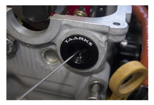
Install the hall sensor into the sensor holder. Leave about 5mm of the sensor sticking out.
