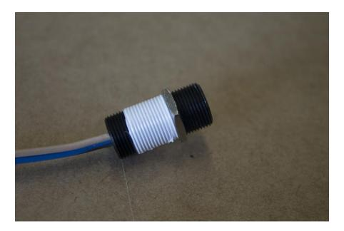
Install the hall sensor holder into the head and tighten the grub screw to secure it in place. Apply a small amount of oil to the o-ring to help it slide in.
