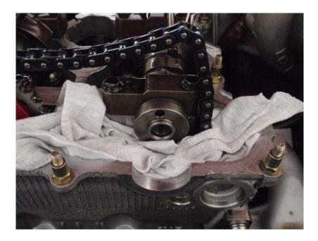
Install the supplied dowel pin into the exhaust camshaft. Note that the tapered end goes in first, as pictured.
