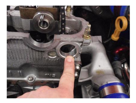
Once the plug has been removed use some 1000 or 1200 grit sand paper to clean any residue out of the hole. Place a rag at the back to stop any dust or debris from falling into the motor.
