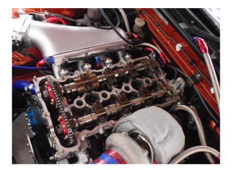
Set the motor to TDC on cylinder one. The lobes on the camshafts for cylinder one will face away from each other.
