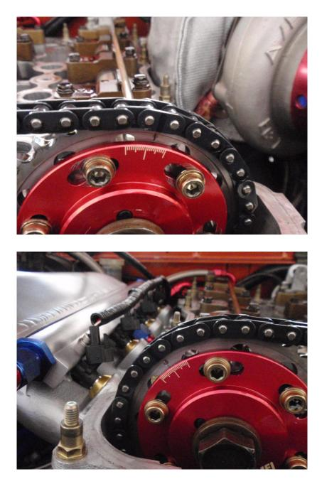
Remove the timing chain tensioner.
