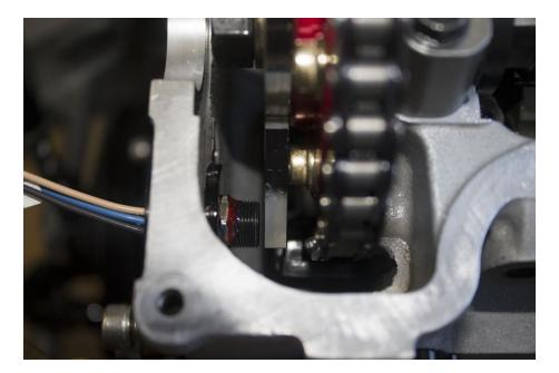
Tighten the locking nut and apply a few drops of high temp Loctite to the threads of the sensor in front of the nut.
