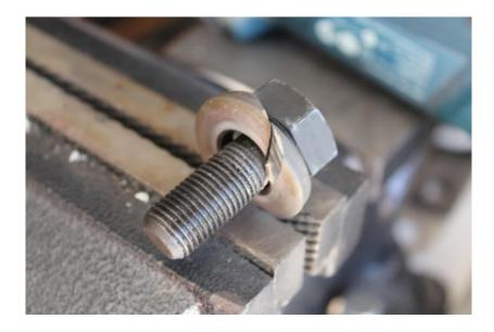
Use a cold chisel or flat blade screw diver and break the washer off. Once removed you will be left with just the bolt.
