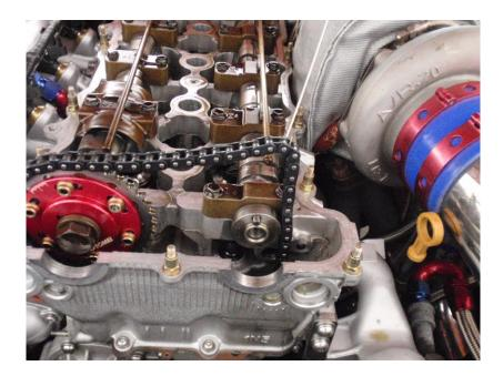
Remove the dowel pin from the exhaust camshaft.
