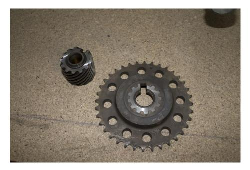
Re-install the cam gear and chain onto the camshaft, make the sure the mark you made earlier on the chain matches the mark on the gear. (Please note that all pictures from here on do not have a chain shown).
