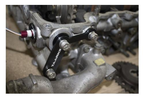
Sensor wiring: Brown: 12v+ Filtered from ECU Blue: GND Black: Signal Output
