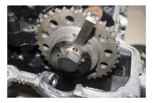
Gently rotate the motor and check for clearance near the old CAS hole, some SR's require a small amount of aluminium casting to be removed. If your head requires this modification you can take this opportunity to mark the casting for removal.
