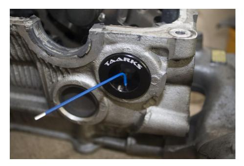
Apply 3-4 turns of thread tape around the sensors thread right after the gap in the thread. Start winding the sensor into the holder so around 10mm is protruding into the head.
