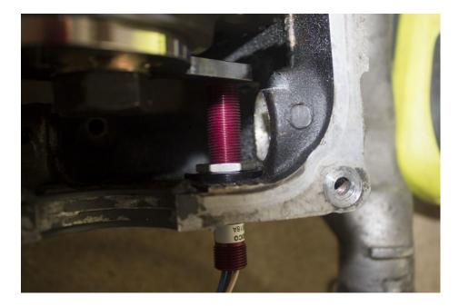
Install the 2 small o-rings onto the cas block off plug and install the plug onto the bracket using the supplied M8 screws.
