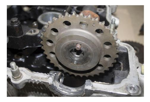
Install the cam sync finger onto the camshaft dowel. Any of the 6 holes can be used. Consult your ECU manufacturer to select the best location for the cam sync to occur in relation to TDC.
