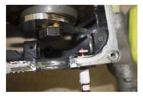
Rotate the engine so the sync finger is in front of the sensor. Continue winding the sensor in by hand until the tip of the sensor is 1 - 1.5mm away from the sync finger, use feeler gauges to confirm the air gap.
