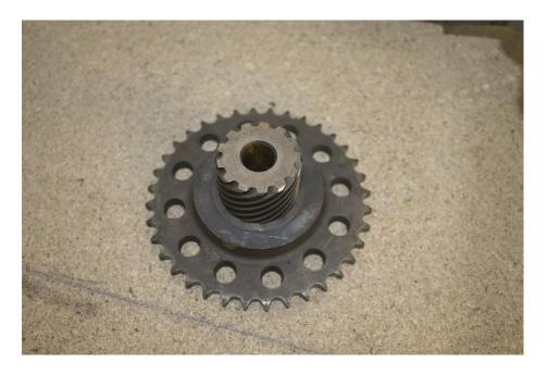
Remove the worm gear from the cam shaft, this is best done in a press.
