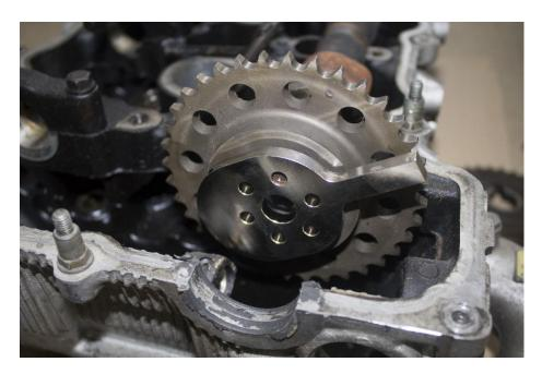
Use the supplied M14 bolt and washer and tighten to spec.
