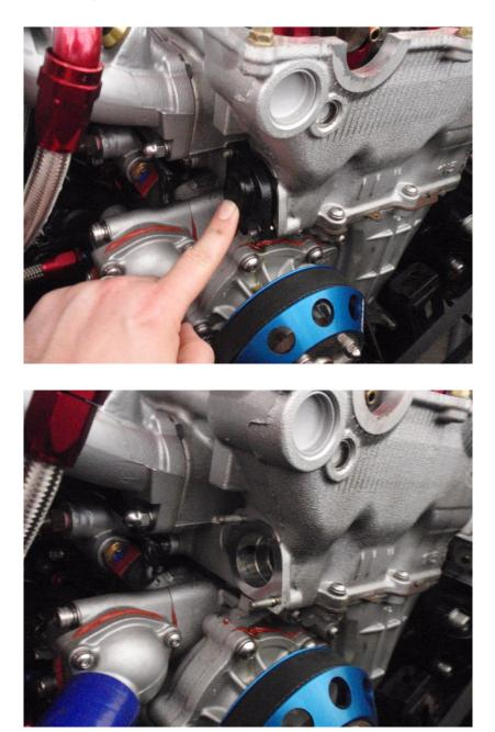
Remove the 24mm bolt from the front of the exhaust camshaft.
