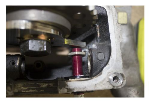
Wind the locking nut back up against the hall sensor holder and tighten, using the feeler gauges confirm the air gap once more. A few drops of the high temp Loctite in front of the locking nut will prevent it coming loose.
