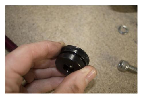
Install the supplied large o-ring onto the holder and then install the holder into the welsch plug hole and use the same 1.5mm allen key to tighten the grub screw securing the holder in place. A small amount of oil on the o-ring will help the holder slide in.
