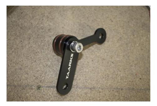
Apply a small amount of oil to the o-rings and install, use the remaining 2 M8 screws to mount the bracket.
