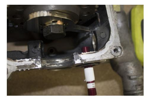
Wind one of the securing nuts supplied with the sensor onto the end of the sensor. Place some rags below the cam gear just in case the nut is dropped during install.
