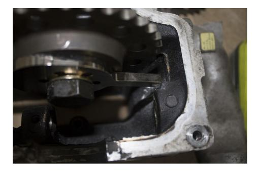
Remove the welsch plug at the front of the head, this can be done by gently taping the plug from behind.
