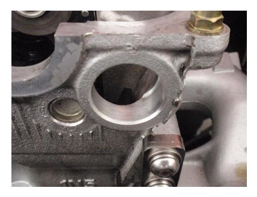
Install the supplied M3 grub screw into the hall sensor holder, this can be tricky and a tip is to install it backwards from the bottom.
