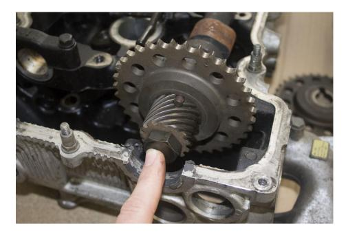
Remove the cam gear from the cam shaft, remember to support the chain and do not let it drop.
