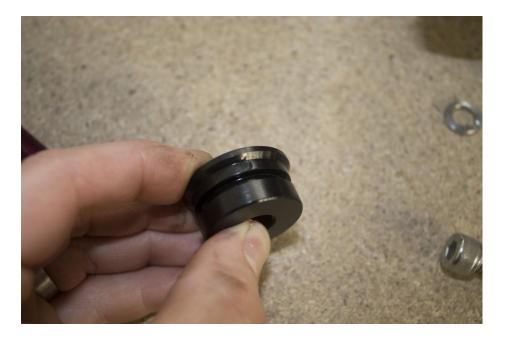
Once you have wound it in as far as you can by hand, use a 1.5mm allen key to continue winding the grub screw in until it is below the surface of the holder.
