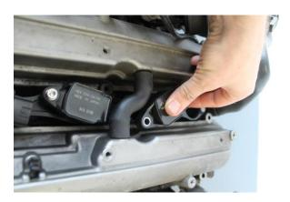
At this point you can install the connectors and wiring loom. It may be necessary to angle the connector to install.
