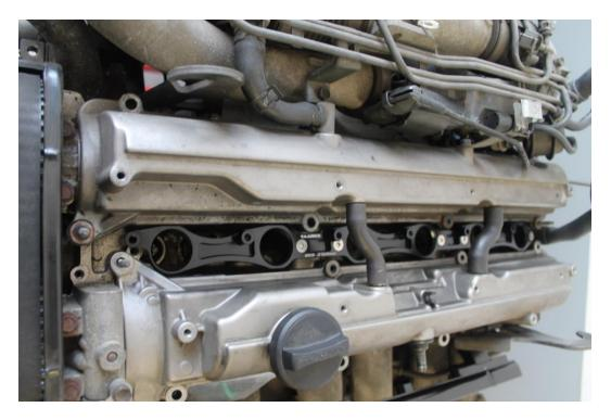
If your engine has a stud at the rear of the motor holding the rocker covers down, the intake side will need to be removed and replaced with the provided M6x30mm cap screw. The stud can be removed using a T4 torx socket or the double nut technique also works.
