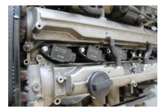
The 4<sup>th</sup> coil will need to be rotated to clear the breather pipe, press the coil down and rotate pack to match the angle of the first 3 coils.
