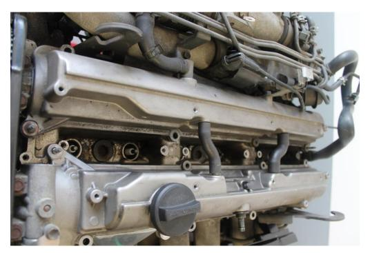
Install the coil bracket using as many of the mounting points as possible. Depending on your engine type you may not be able to use every bolt. It may be necessary to loosen the rocker cover bolts and lift the rocker covers to get the bracket into the valley.
