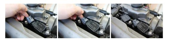
The last coil will need to have the connector installed just before pushing the coil down onto the bracket.
