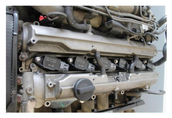
Note: It is recommended to run Resistor type spark plugs with these coils, running non resistor plugs can damage the coils.
