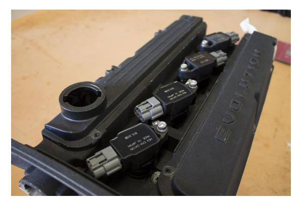
Use the supplied M6 bolts and spring washers to bolt the coils onto the bracket.
