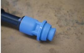
Install the coils onto the bracket by gently pushing down, make sure not to pinch the rubber boot of the coil as it seats onto the bracket.
