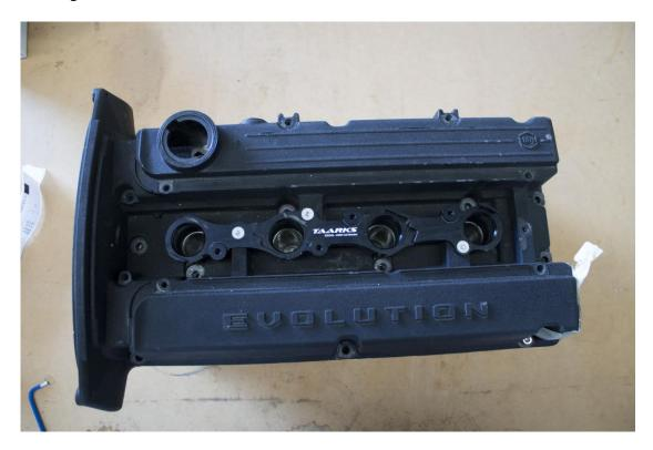
Now it's time to install the coils. The coils have already been modified with new boots and springs ready to go. On each of the coils use a small amount of the supplied dielectric grease on the inside of the coil boot where the spark plug enters, this helps the boot slide on and off the spark plug easier. Also apply a small amount to the largest diameter flange on the boot.
