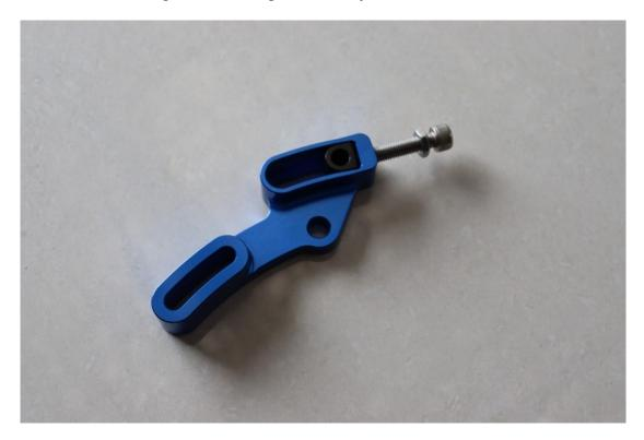
Install the adjuster onto the factory alternator mount. Ensure that the split washer is installed onto the M8 bolt followed by the flat washer as pictured below. The supplied spacers are installed between the adjuster and factory alternator mount. Only hand tighten the bolts.
