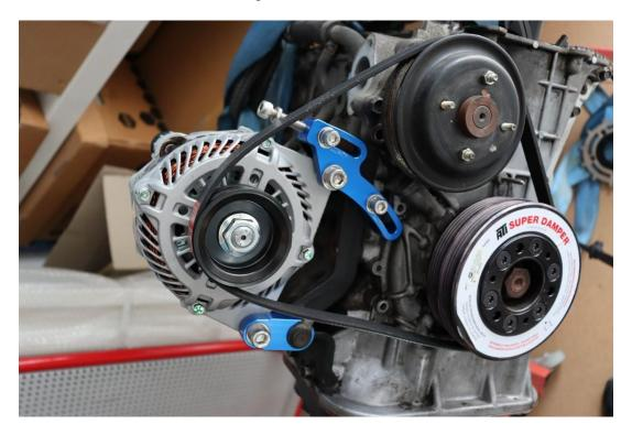
Start screwing the adjuster bolt in to tighten the belt. Use the specifications from the service manual on the next page, 7-8mm deflection at the point indicated with a force of 10kg with the appropriate tool.
