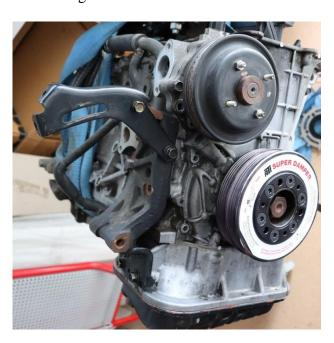
Remove the factory alternator adjuster bracket.
