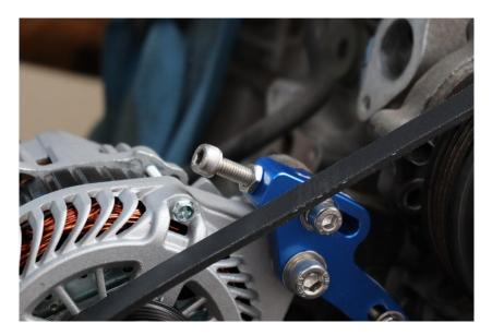
Tighten all the remaining bolts. And re-check the belt tension. Adjust again if necessary.
