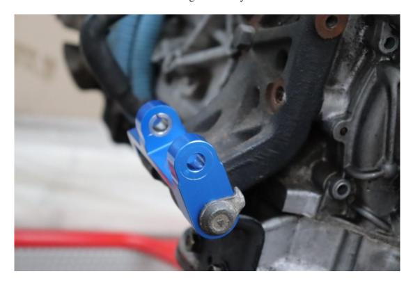
Assemble the alternator adjuster bracket as shown below. The black adjust sleeve will only work one way, slide it back and forth to ensure it moves easily. Use the M8 bolt that is threaded along it's entire length for the adjuster bolt.
