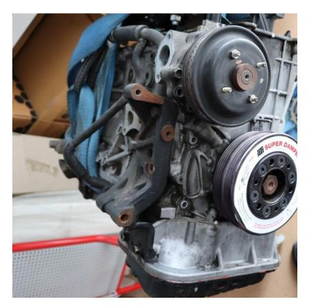
Install the lower alternator bracket using the factory alternator bolt and nut.
