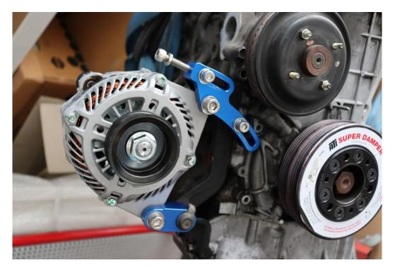
Install the new fan belt onto the engine/alternator.
