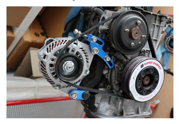
Start screwing the adjuster bolt in to tighten the belt.
