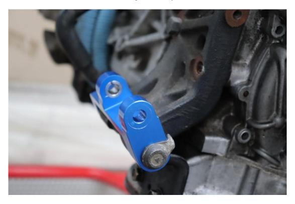
Assemble the alternator adjuster bracket as shown below. The black adjust sleeve will only work one way, slide it back and forth to ensure it moves easily. Use the M8 bolt that is threaded along it's entire length for the adjuster bolt.
