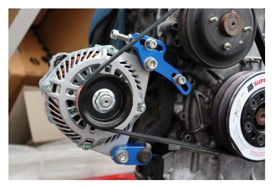
Re-install the power steering, A/C belts and electrical connectors to the alternator.
