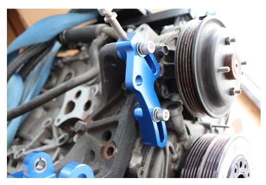
Using the supplied M10x90mm bolt and M10 flat washer install the LS1 alternator onto the lower mount. Once installed another M10 flat washer and M10 nyloc nut is used to secure the bolt. Hand tighten only.
