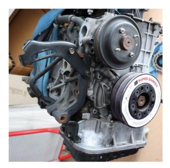
Remove the factory alternator adjuster bracket.
