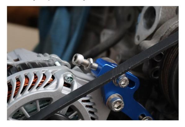
Once the desired tensioner is reached tighten the locking nut in place.
