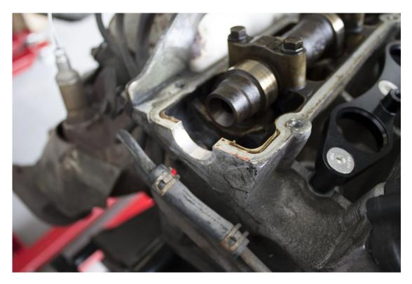
Clean any old gasket goo, oil etc from the head in the half moon area and on the front and rear surfaces. Do a final wipe over with acetone or wax & grease remover.
