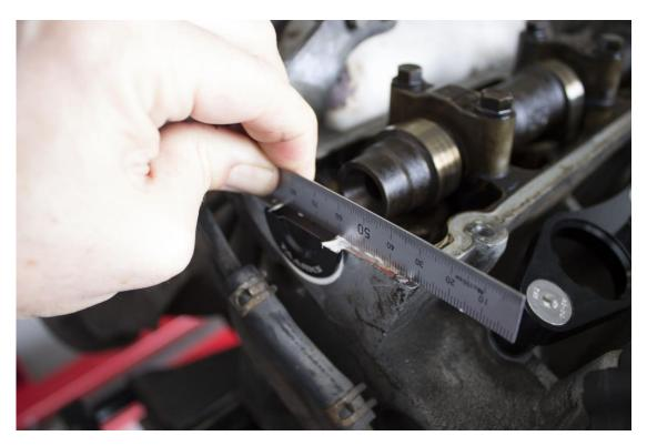
Leave the liquid gasket maker to dry and remove any excess with a knife blade or similar.
