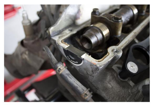
Using a steel ruler or similar straight edge push the seal down until it sits level with the head. The more time and care taken during these steps the better the result.
