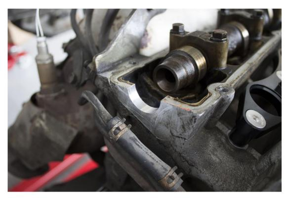
Apply a 3mm bead of liquid gasket maker to the head.
