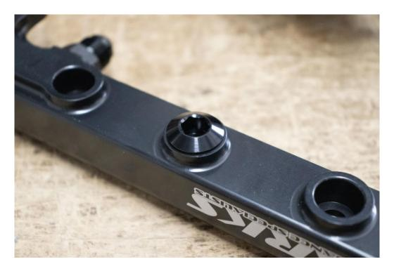
Apply a small amount of engine oil to the injector o-rings and press them into the fuel rail.
