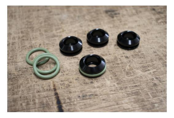
Remove the factory rubber insulators from the intake runners. Lubricate the o-ring of the injector adapters with small amount of engine oil and press the adapters into the intake manifold.
