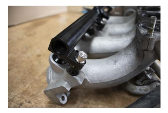
Install the o-rings on the AN fittings and lubricate with a small amount of engine oil, install them into the ends of the fuel rail. Do not over tighten, nipped up is fine.
