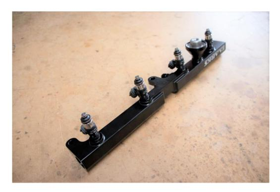
The kit is supplied with 3 different height fuel rail mounts, the shortest goes in the middle, the longest towards the front of the car and medium towards the firewall.
