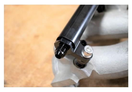
This kit is supplied with new injector connectors that will need to be crimped onto your existing wiring loom. We recommended having this done by an Auto Electrician.
