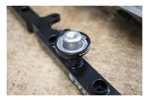
If you do not want to run the fuel pulse damper block the port off with the supplied AN6 plug, lubricate the o-ring with a small amount of engine oil. An 8mm allen key is required.
