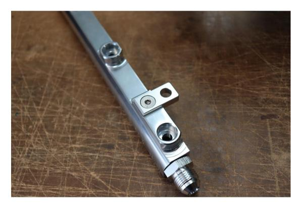
If the centre return port is not being used them install the supplied block off plugs as shown below.
