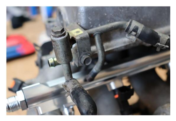
Crimp the new connectors onto your existing wiring loom, plumb new fuel lines into the rail and re-install the upper plenum chamber and cross over pipe etc.
