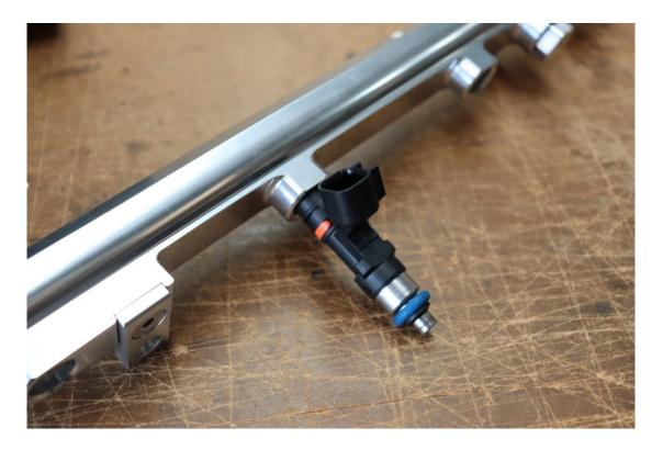
Lubricate the O-rings on the other end of the injectors and push the injectors into the injector adapters that you installed into the intake manifold earlier.
