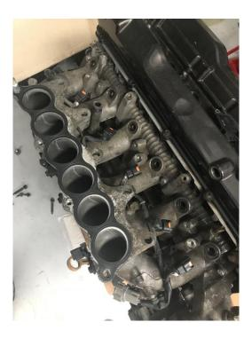
Remove the standard rubber injector insulators.
