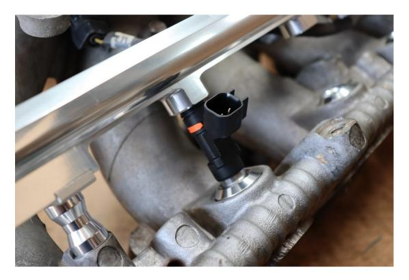
Use the supplied short M8 bolts, spring washer and short fuel rail mount to secure the fuel rail to the intake manifold.
