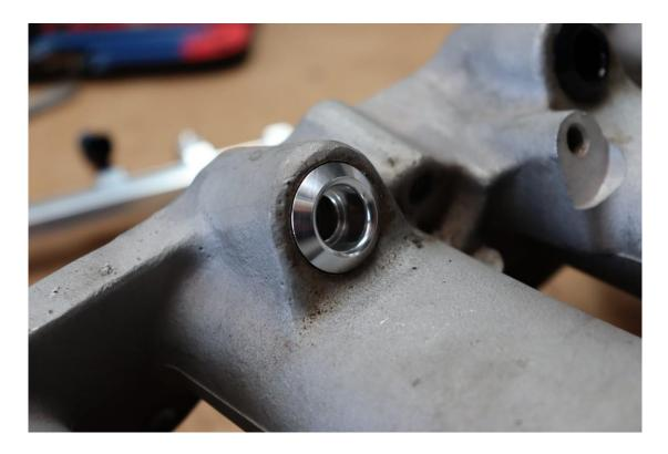
Attach the fuel rail mounts onto the fuel rail using the supplied M6 counter sunk screws. A 4mm allen key is required. A small amount of Loctite on the threads is recommended.
