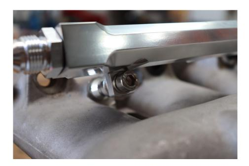
If your intake manifold has not been machined correctly and requires packers it's recommended to put them in between the fuel rail and fuel rail mount as pictured below.
