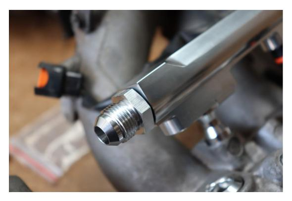
Crimp the new connectors onto your existing wiring loom, plumb new fuel lines into the rail etc.
