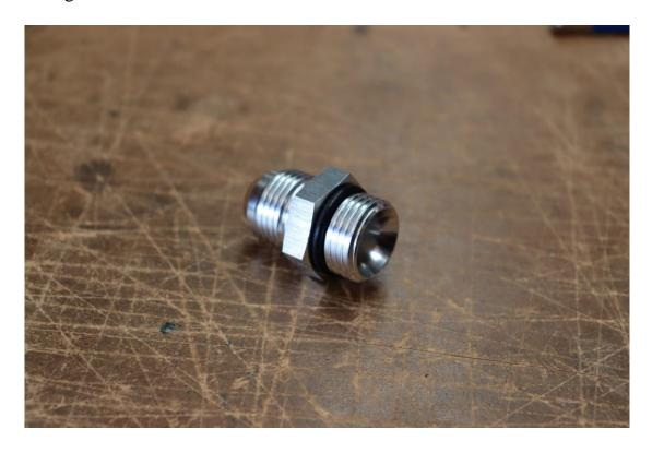
Screw the AN adapters into the ends of the fuel. Do not use any thread tape or sealant on the threads.
