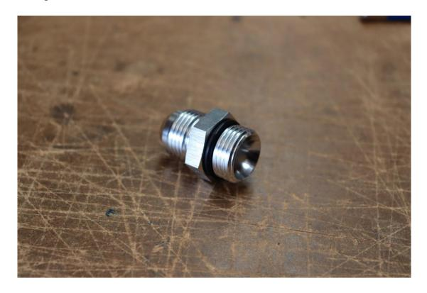
Screw the AN adapters into the ends of the fuel. Do not use any thread tape or sealant on the threads.
