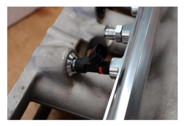
If you are using ¾ length injectors use the supplied short M8 bolts, spring washer and short fuel rail mount to secure the fuel rail to the intake manifold.
