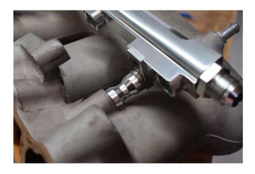
Select either the AN6 or AN8 adapters to use on the fuel rail, install the o-rings as shown below.
