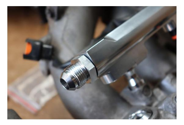
The standard coolant bleed nipple may need to be adjusted to clear the new fuel rail, either by bending the metal lines slightly or unbolting it from the intake plenum.
