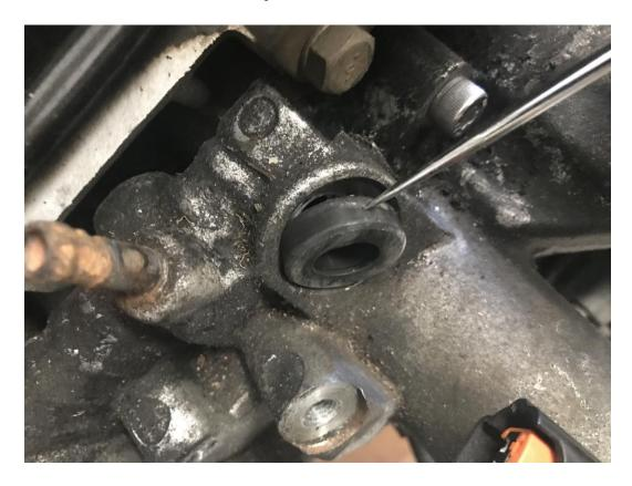
Install the injector adapters into the intake manifolds, lubricate the Orings with a small amount of oil to help them push in.
