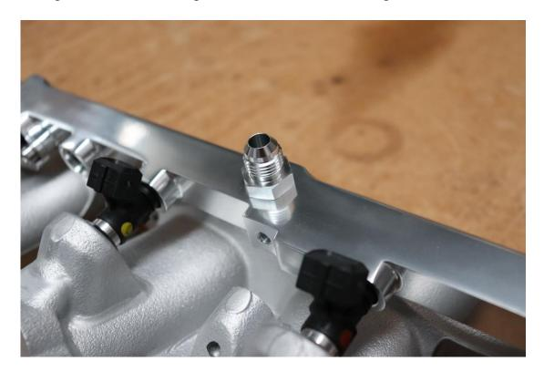
If you are not planning to use the center return port you can block if off with the supplied AN6 plug, lubricate the o-ring with a small amount of engine oil. An 8mm allen key is required.
