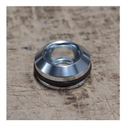
Lubricate the o-ring with small amount of engine oil and press the adapters into the intake manifold.
