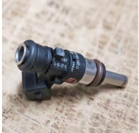
Apply a small amount of engine oil to the injector o-rings and press them into the injector adapters. Ensure the connector face up.
