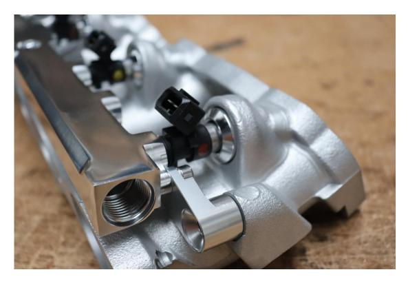
Using the supplied M8 countersunk bolts bolt the rail onto the intake. A 6mm allen key is required.
