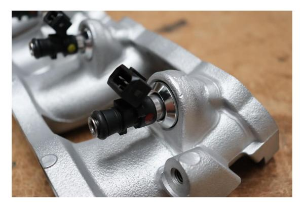
Lubricate the upper o-rings with a small amount of engine oil and press the fuel rail onto the injectors.
