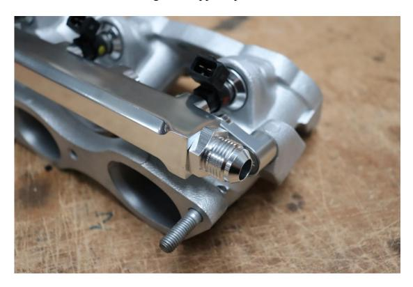
If you are planning to use the center return port install the supplied AN6 fitting, lubricate the o-ring with a small amount of engine oil.
