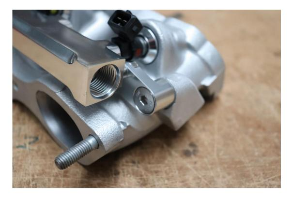
Choose either the AN6 or AN8 supplied fittings, install and lubricate the o-rings with a small amount of engine oil and install them into the ends of the fuel rail. Do not over tighten, nipped up is fine.
