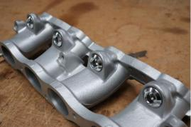
Some injectors like the bosch 980cc injectors will need the locator trimmed slightly to clear. Not all injectors have these locators. Trim 2mm off the locator as shown below. (this only needs to be done for injector 1 & 4).
