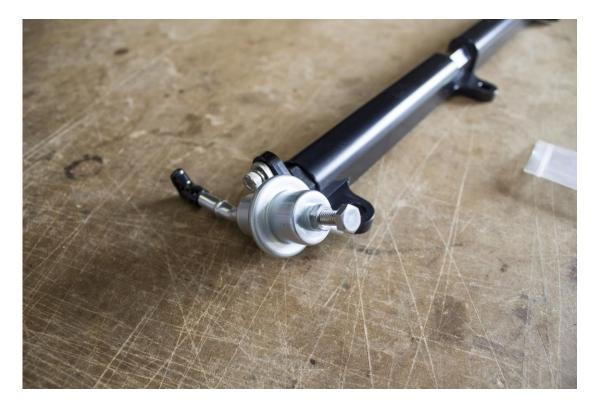
Use the supplied M5 allen key bolts and spring washers to mount. Before tightening the M5 bolts make sure to rotate the fuel pressure regulator to the desired angle.
