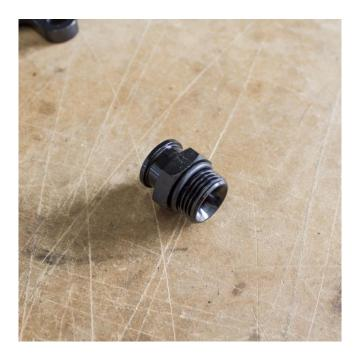
Lubricate and install the o-ringed fitting into the end of the fuel rail.
