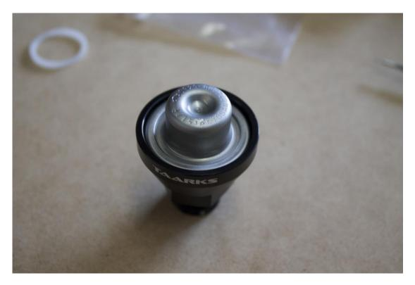
While pressing the damper down install the circlip into the circlip groove.
