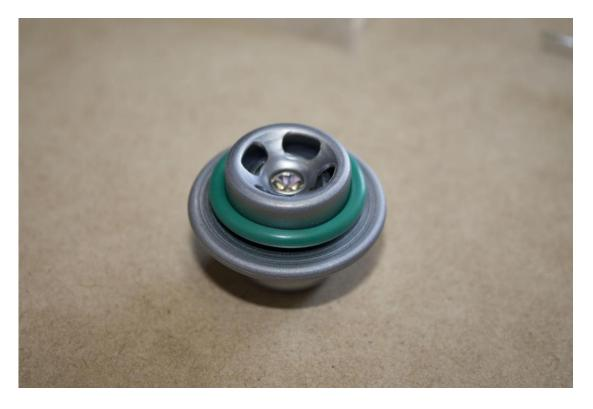
Lubricate the o-ring and install the damper into the housing.
