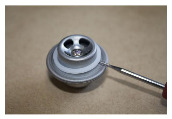
Install the supplier o-ring onto the fuel pulse damper.
