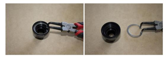
Remove the white plastic ring from the fuel pulse damper.
