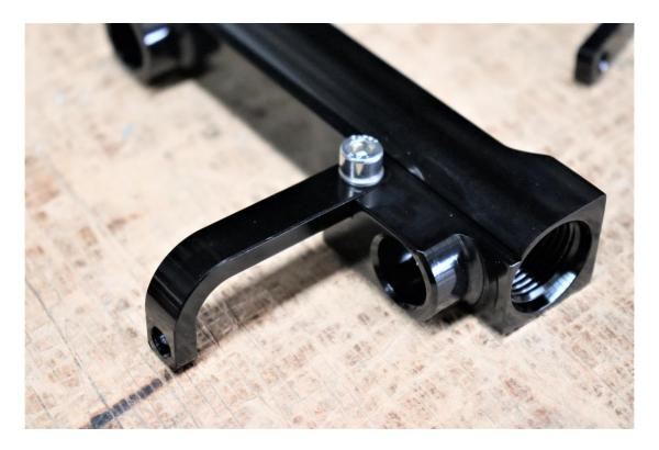
This fuel rail has a center return port allowing you to dual feed the rail. Fit either the AN6 adapter if you are using the center return port or install AN6 plug if you do not want to use the center port. Install the o-ring to the fitting you are using and apply a small amount of engine oil to the o-ring before installing.
