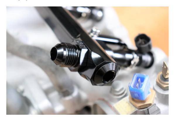
All that's left to do is wire up your injectors and plumb up the fuel lines.
