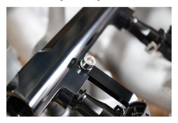
The fuel rail is supplied with AN6 and AN8 adapters for the rail. Select the size you are going to run and install the o-rings to the fittings.
