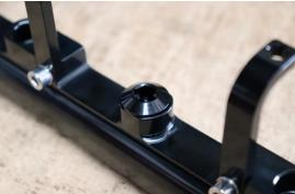
Lubricate the o-rings of your injectors with a small amount of engine oil and fit them to the fuel rail.
