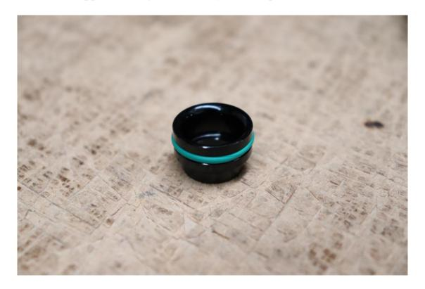
Lubricate the o-ring with a small amount of engine oil and gently press them into the intake manifold making sure the o-ring does not get pinched.
