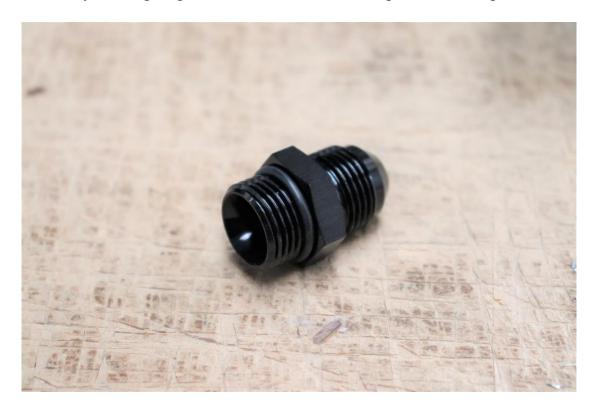
Apply a small amount of engine oil to the o-rings and install them onto the fuel rail. The rear fitting is installed into the end of the fuel rail, the front fitting is installed into the top of the fuel rail. Install the supplied AN8 plug into the front of the fuel rail as shown below.
