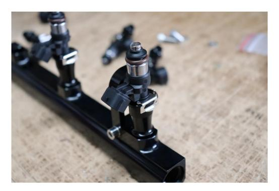
Lubricate the nozzle end o-rings of your injectors with a small amount of engine oil and fit the rail and injectors to the intake manifold. Take care in guiding each injector into their respective injector adapter.
