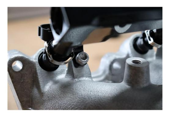
Once the M6 bolts are tight it's time to tighten the M5 bolts on the rail.
