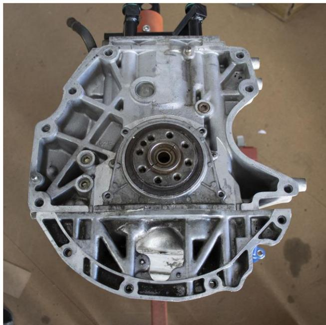
Test fit the adapter plate onto the engine and ensure the engine block dowels do not protrude past the adapter plate surface. If they do they will need to be filed down.
