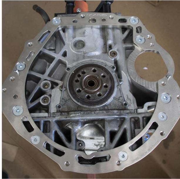
The starter motor bolt holes are currently threaded, these holes need to be drilled out to 10.5mm
