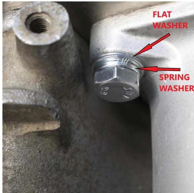
Once the starter motor is installed check the bolts do not protrude past the surface of the adapter plate, if they do the bolts will need to be removed and filed down.
