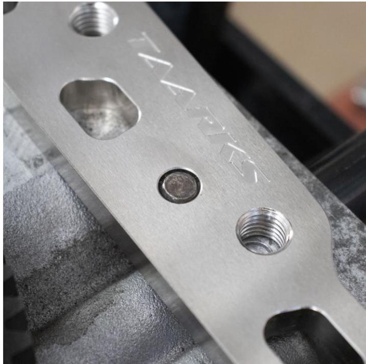
Install the adapter plate onto the engine using the supplied countersunk bolts. Note the head on one of the M12 countersunk bolts has been machined down to fit the hole next to the gearbox dowel.
