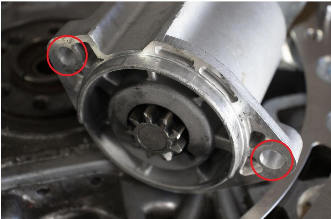
Once drilled the starter motor can be installed using the supplied M10x30mm hex head bolts. Ensure the spring washer and flat washer are installed as shown below.
