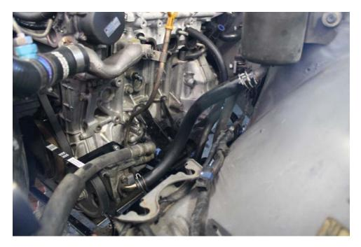
Re-fill the reservoir with power steering fluid.
