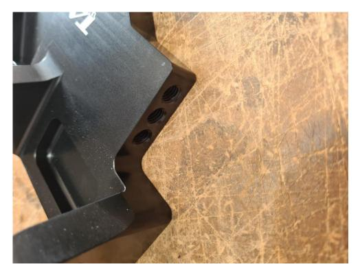
Once adjusted tighten the main bolt and lock the adjuster with the locking nuts.
