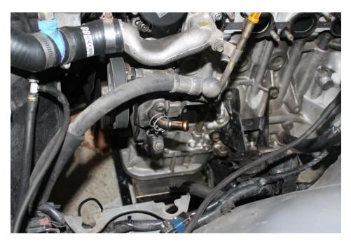
Loosen the tensioner on the power steering pump bracket and remove the belt.
