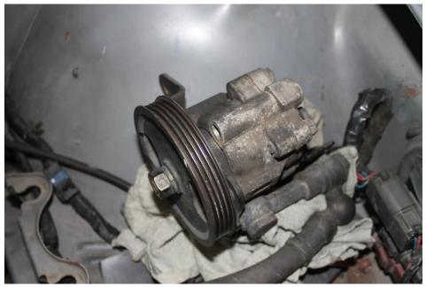
Remove the power steering mount from the engine block.
