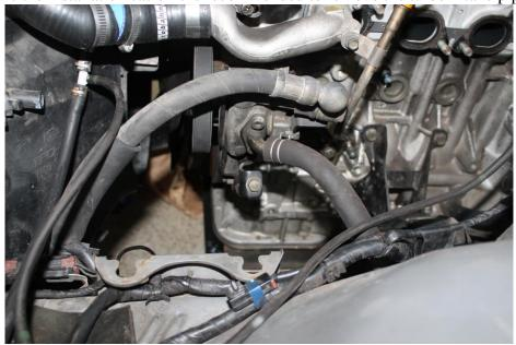
Remove the power steering feed line from the pump and drain the power steering fluid from the system. This can be a messy job, so have a drain tray under the car and lots of rags.
