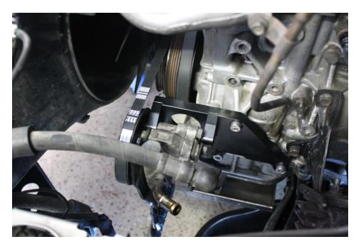
While holding the pump up and using the supplied M8x25mm long bolt, split washer and washer, bolt the adjuster onto the bracket.
