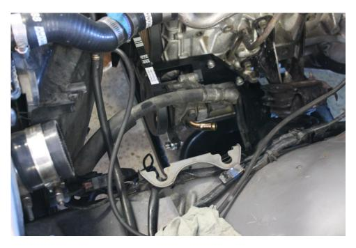
Install the supplied rubber hose onto the pump and cut to length. Use the original hose clamps.
