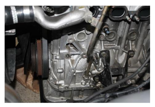
Using the 3 supplied M10 bolts and split washers install the bracket onto the engine block.
