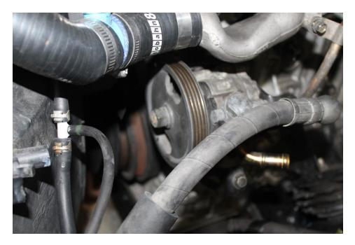
Remove all the bolts holding the pump onto the bracket and move the pump off to one side. Do not remove the pump from the high pressure line.
