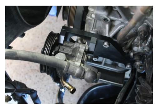
Push the pump down as low as it will go and slip the belt onto the pulleys. If you are not able to slip the belt on, remove the pulley from the pump and re-install the pulley with the belt at the same time.
