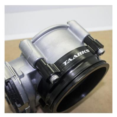
Lastly, install the thick o-ring into the o-ring grove on the adapter. The throttle body is now ready to be installed.
