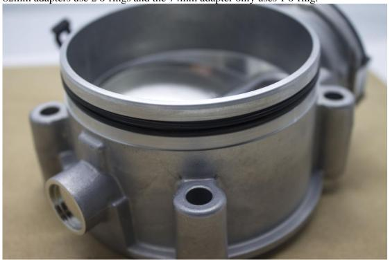
Apply a small amount of lubricant to the o-rings and side the adapter onto the throttle body. Align the mounting holes on the adapter to the mounting holes on the throttle body.
