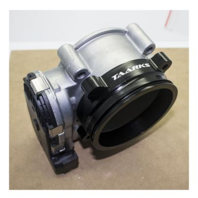
Place the spacers in between the adapter and throttle body, insert the M6 bolts through.
