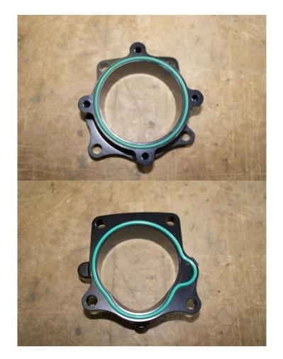
Install the adapter onto the intake manifold using the supplied M8 bolts and spring washers.
