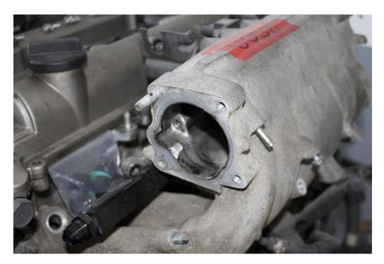
Remove the 2 studs from the intake manifold.
