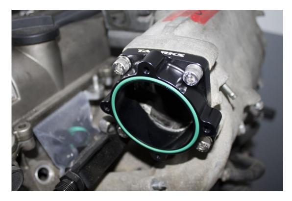
Next install your 68mm bosch throttle body onto the adapter.
