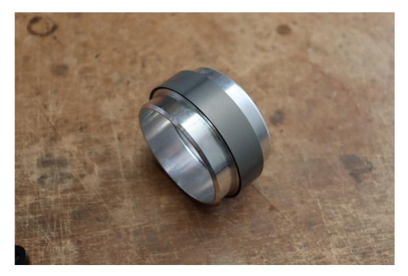
Install the clamp over the internal ring and re-install the M6 bolt and nut. From factory the bolts have a small amount of anti-seize applied to them. If the clamp needs to be removed re-apply a small amount of anti-seize to the bolts. Tighten bolt M6 bolts.
