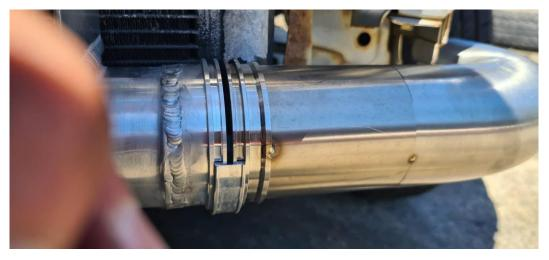
Re-install the o-rings and apply a thin coating of o-ring or silicone grease to the o-rings.
