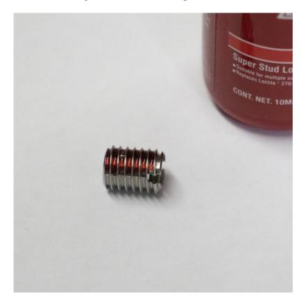
Using a flat head screw driver wind the thread adapters into the intake manifold as shown below.
