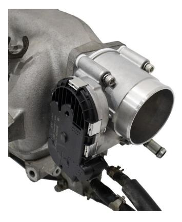
From here the throttle body will need to be wired into your aftermarket ECU (a pinout can be found below). The intercooler pipe may also need to be modified to suit the new throttle body.
