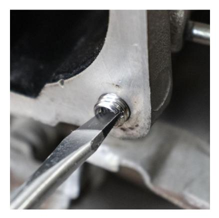
Ensure the thread adapters are flush or just below the surface of the intake manifold as shown below. Allow 24 hours for the Loctite to cure before moving onto the next step.
