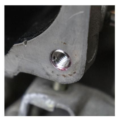
Once the Loctite has had 24 hours to cure you can now install the throttle body using the supplied M6 bolts and spring washers.
