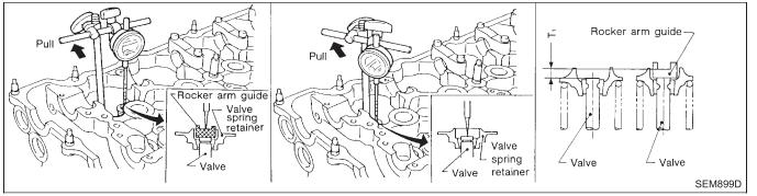
Make sure that the following parts are installed to the cylinder head: valve, valve spring, collet, retainer, and rocker arm guide (except shim). Measure difference (T<sub>1</sub>) between contact surfaces of rocker arm guide and valve stem end on shim side. When measuring, lightly pull dial indicator rod toward you to eliminate play in Tool (KV10115700).
