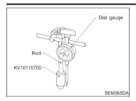
Install Tool\* into hydraulic lash adjuster fixing hole. \* Tool (KV10115700) is screwed into magnetic stand rod used with dial gauge.
